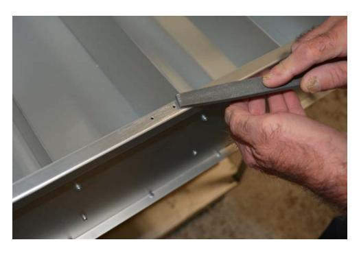
Remove broken roller catch and flat file off any remaining burrs
