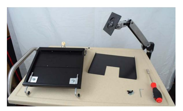
3. Connect the tray to the VESA plate using the 4 x 8-32 button head bolts, keps nuts, and hex tool provided. 11/32" Nut driver not included.
