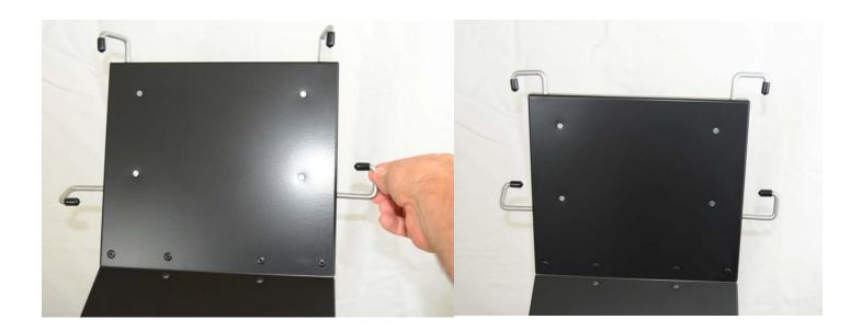
4. Open the laptop and position the leading edge of the keyboard under the front two rods.
