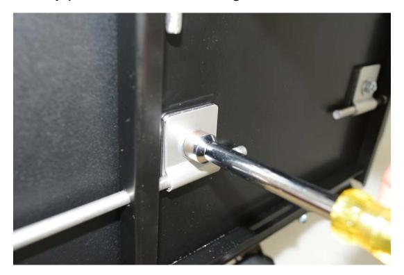
2. Rotate the 4 rods on top so that they do not impede the screen from sitting flush against the upper section of the tray.
